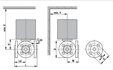
X/Y: Minimum distance with respect to the valve centre.
